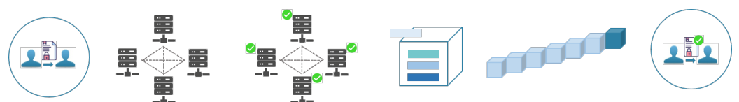
Figure 1. Blockchain transaction processing: (1) Transaction request, (2) Transaction broadcast to P2P network nodes, (3) Transaction verification using consensus algorithms, (4) Transaction packed into block with other transactions, (5) The block added to the blockchain, (6) Transaction completed
